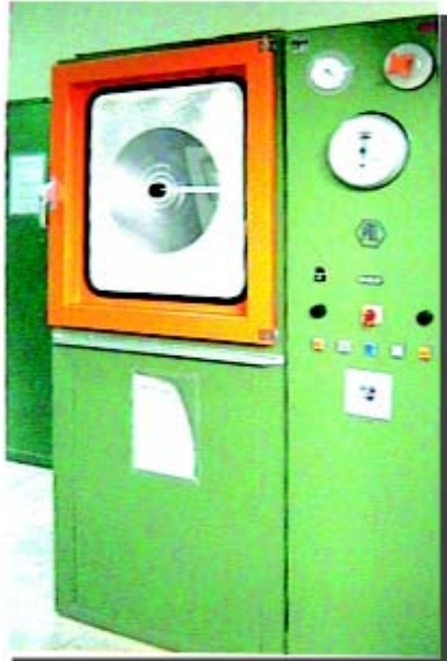
Dust Proof Testing Unit ( I P Test )
