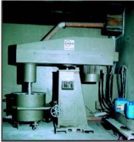
Resin Mixing Unit
